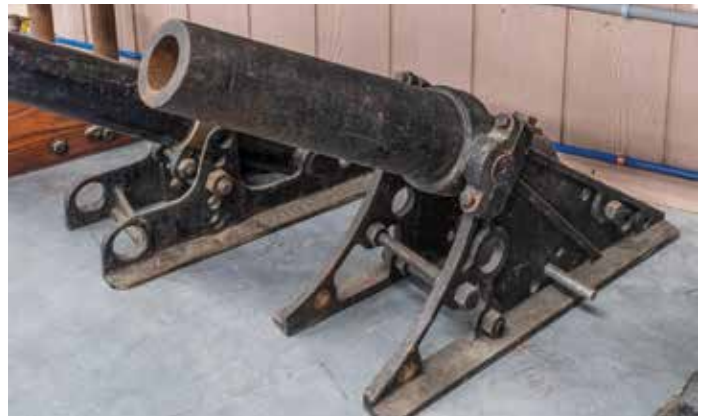
Lyle line throwing guns were used to throw lines between ships, and were required on all ships that handled passengers.
