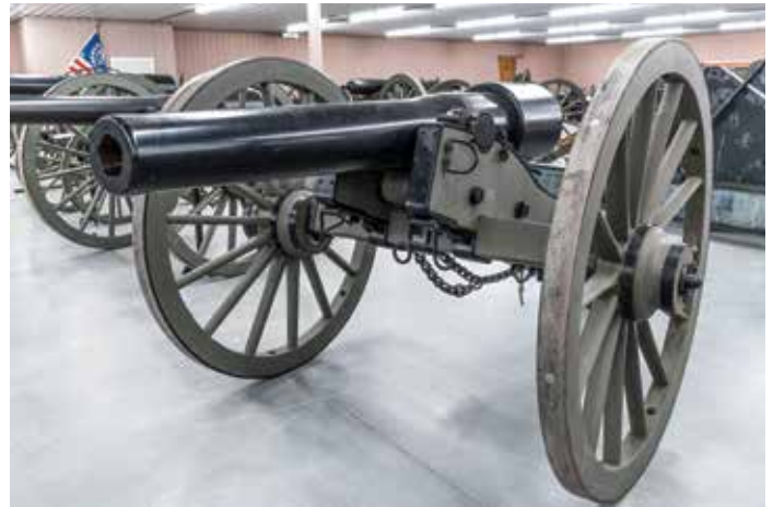
This 20-pounder Navy Parrott Rifle, serial #325, was manufactured in 1865 at West Point Foundry, weighs 1,710 pounds, and still has its original rifled bore.
