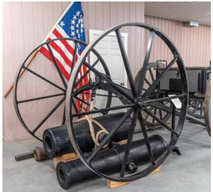
Smithgall has used this reproduction hand sling cart to move his 10-inch siege mortar. The heavy item to be moved is slung under the axle of the cart, suspended by a chain or heavy rope.
