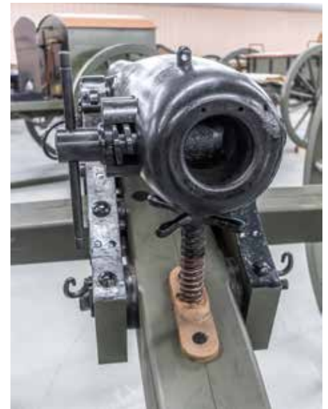
The breech of an experimental 3.2-inch model ordnance rifle with a Krupp type breech is serial #3 of only five manufactured to develop the 3.2-inch breechloading rifle.
