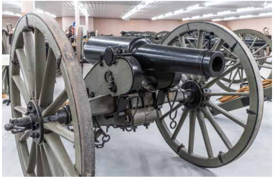
This 3.67-inch (12-pounder) Wiard rifle, serial #61 was manufactured in 1862 at O'Donnell Foundry in New York, N.Y. When mounted on the innovative Wiard carriages, these guns could be elevated up to an angle of 35 degrees, allowing them to fire with a trajectory more like mortars.
