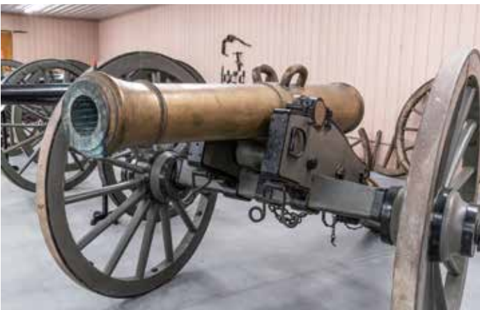
This bronze 12-pounder Model 1841, serial #56, is rifled with the James system of rifling. It was manufactured in 1854 by Ames Manufacturing Company. It weighs 1,773 pounds and fired a service charge of 2.5 pounds.
